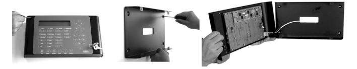
Figure 13 - Mounting a Repeater
