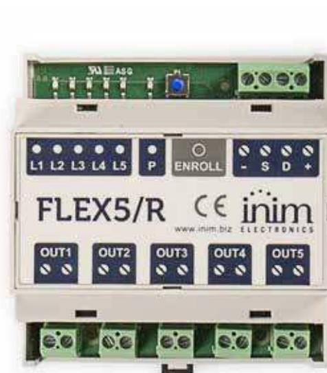
Flex5/R is a BUS module with 5 relays, each relay output can control, through configurations programmed via the control panel, both AC and DC loads up to a maximum of 16A and allows, even locally, to check the status of the individual outputs. The device is designed for installation on a 5-module DIN rail. These characteristics make it particularly suitable for home-automation applications.
