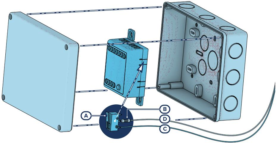
The peripherals with visible terminals and which do not have an anti-tamper device can still be equipped with protection by intervening on the assembly procedure.
