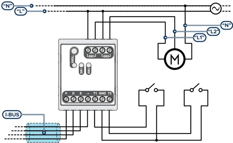
For this operating mode it is necessary to connect two buttons to terminals 'T1' and 'T2', respectively for driving the roller shutter up or down. We recommend a double or tilting pushbutton panel, with mechanical interlock, specially designed for roller shutters.
