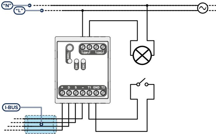
For this operating mode, a switch/button must be connected to terminal 'T1' in order to control the light point. Terminal 'SW1' must be connected to the light point that is to be controlled.
