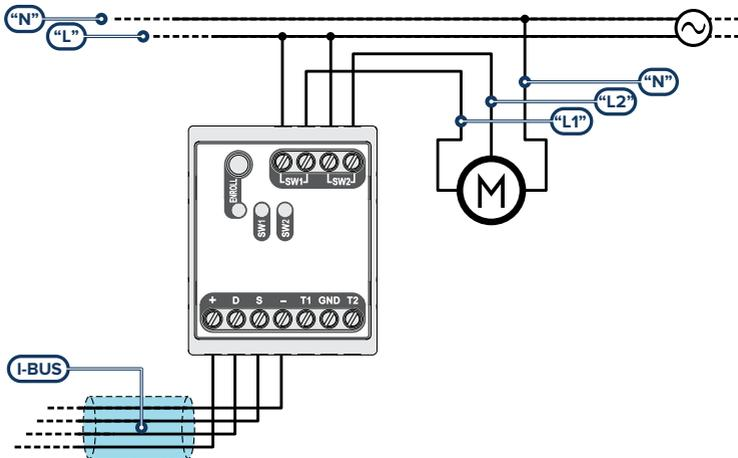
For this operating mode it is necessary to connect terminals 'SW1' and 'SW2' respectively to the up and down phases of the roller shutter.
