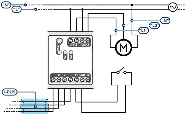
For this operating mode, a single button must be connected to terminal 'T1' in order to drive the roller shutter.
