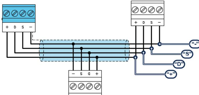
The peripheral devices of Inim Electronics control panels are to be connected to the control panel via the I-BUS.
