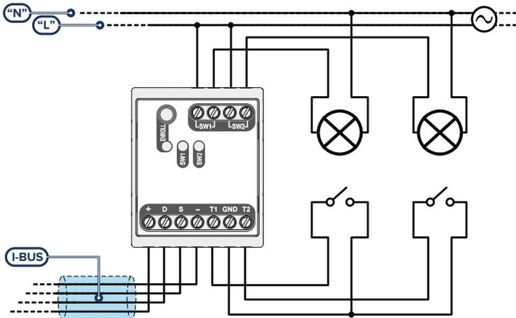
For this operating mode, it is necessary to connect two switches/buttons to terminals 'T1' and 'T2' respectively to control the light points connected to terminals 'SW1' and 'SW2'.
