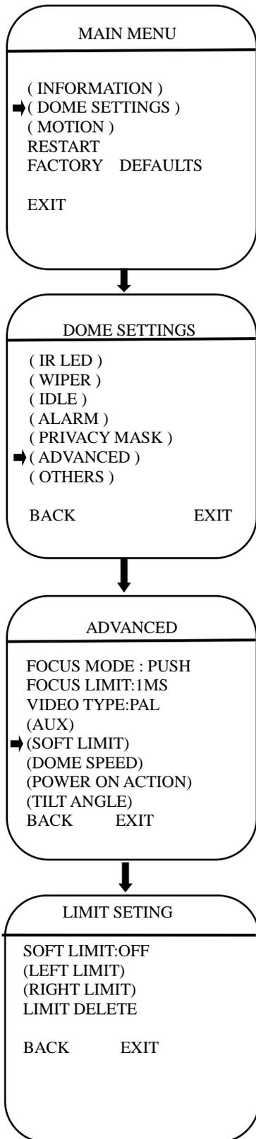
The user can set up the soft limit to define the left and right boundaries for the pan movement.
