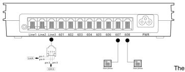
system provide door opener(door-open switch, connect with the wire of electric lock) interface, and system can defined two extension as door phone.
