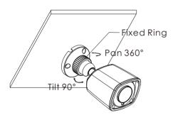
5 Tighten the fixed ring after the adjustment.
