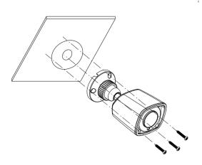
④ Bracket adjustment. Before adjustment, preview the image of the camera on a monitor and then loosen the fixed ring to adjust the view angle of the camera.
