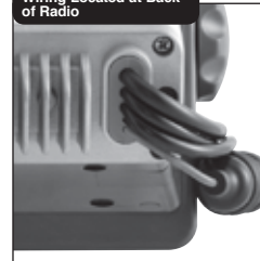
Wiring Located at Back of Radio
