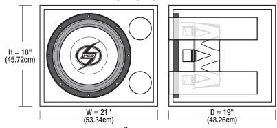
Small Vented 2.75ft<sup>3</sup> (77.9L), Ports (2) 4"x20.75" **Optimal Vented 3.25ft<sup>3</sup> (92.0L), Ports (2) 4"x15.75"**Large Vented 4.5ft<sup>3</sup> (127.4L), Ports (3) 4"x16"
