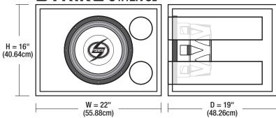
Small Vented 2.5ft<sup>3</sup> (70.8L), Ports (2) 3"x10.5" **Optimal Vented 3.0ft<sup>3</sup> (84.9L), Ports (2) 4"x16.5"**Large Vented 4.25ft<sup>3</sup> (120.3L), Ports (2) 4"x9.5"
