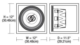
Small Sealed 0.40ft<sup>3</sup> (11.3L) **Optimal Sealed 0.65ft<sup>3</sup> (18.4L)**Large Sealed 1.0ft<sup>3</sup> (28.3L)
