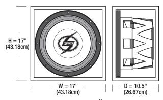
Small Sealed 1.0ft<sup>3</sup> (28.3L) **Optimal Sealed 1.25ft<sup>3</sup> (35.4L)**Large Sealed 2.0ft<sup>3</sup> (56.6L)
