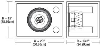
Small Vented 1.5ft<sup>3</sup> (42.5L), Ports (2) 2.5"x13.25" **Optimal Vented 1.75ft<sup>3</sup> (49.6L), Ports (2) 2.5"x10.75"**Large Vented 2.5ft<sup>3</sup> (70.8L), Ports (2) 2.5"x6.5"
