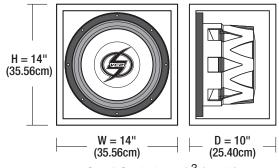
Small Sealed 0.60ft<sup>3</sup> (17.0L) **Optimal Sealed 0.75ft<sup>3</sup> (21.2L)**Large Sealed 1.25ft<sup>3</sup> (35.4L)
