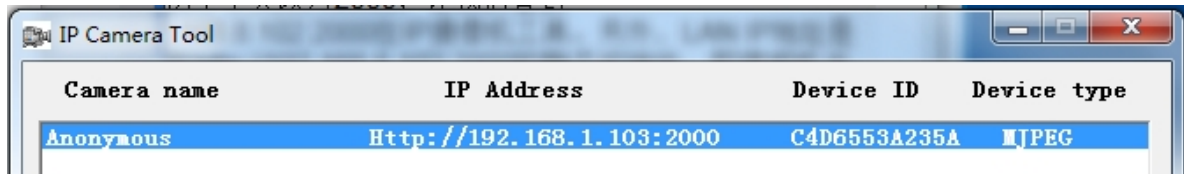
Static IP address and port 2000 set in IP Camera Tool
