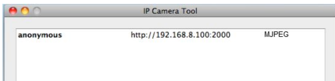
Static IP address and port 2000 set in IP Camera Tool
